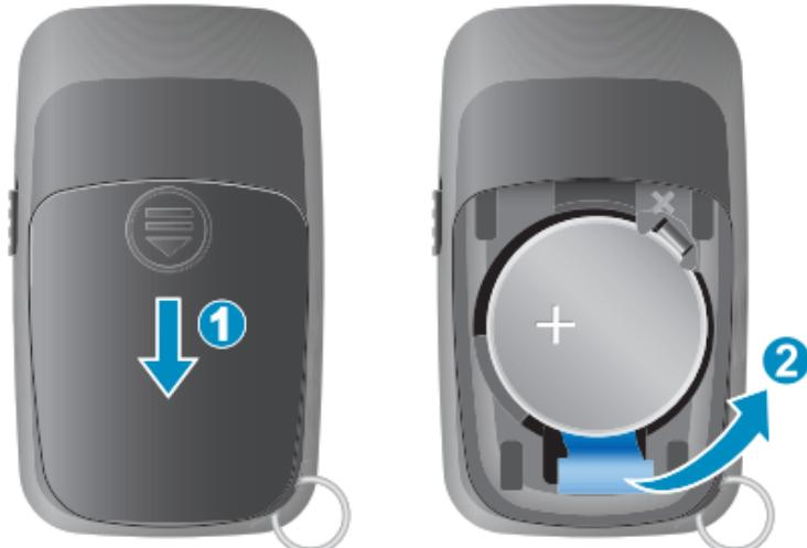
**Insert the battery with the "+" symbol facing up:**
